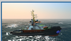
Anchor points are shown with a blue sphere at the bow.
