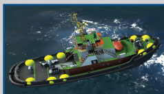
Mooring lines connection points are shown as yellow spheres.
