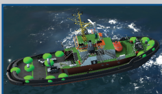
Tow line connection points are visible as green spheres.
